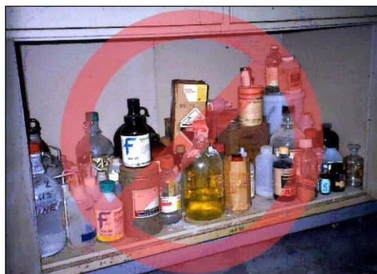
Figure 6.2 – Improper Fume Hood Storage
