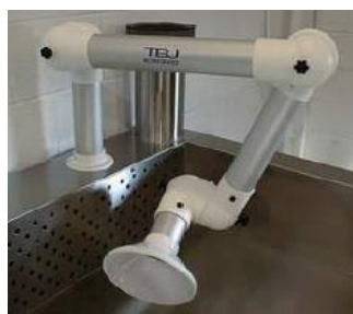
Figure 5.7 – Examples of Snorkels and Canopy Hoods
